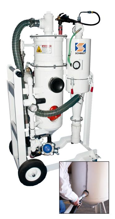
The Schmidt miniBRS is a compact and easily maneuverable abrasive blasting system that blasts and then recovers spent abrasive, contaminants and dust in the same step, eliminating the need for containment. The system can also be used to blast and then vacuum abrasive independently.
