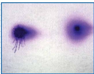
Fig 10: Haste makes waste. Slow down. Moving the airbrush while spraying will make dots into dagger strokes. Keep the air on, and exercise good paint control.
