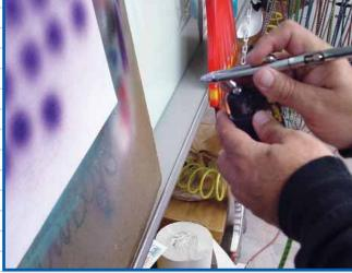
Fig 8: Here I've moved back to four or six inches from the paint surface. I'm keeping the air constant and pulling back all the way on the trigger, then rolling the trigger forward again. This makes bigger, well-formed dots. Notice that distance also equals softness of the dots' outlines.
