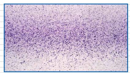
Fig 3: An example of "tip dry." It only takes a small amount of paint dried on the needle to adversely affect proper airflow and atomization of the paint.
