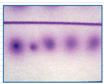
Fig 11: Not enough paint. The airbrush nozzle was too far away from the surface as well. These dots are too subtle and are turning into fuzzy shaded areas.
