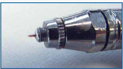
Fig 4: An example of a properly cleaned needle. Note that the nozzle, or needle cap, has been removed for cleaning. Gently unscrew the nozzle and treat these small parts, particularly the needle, carefully. Even slight damage can make your paint go haywire. A soft cloth or tissue wetted with cleaning solution, or very gentle scraping with a fingernail, can remove dry paint from the needle tip. But again, go slowly and exercise
