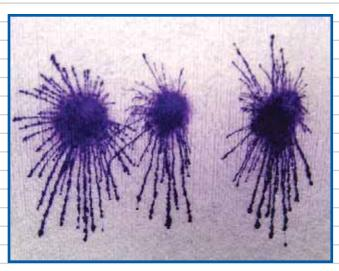
Fig 9: Here's a common error—spidering. This happens when you shoot too much paint, your air pressure is too high, your paint is too thin, or some combination of these. This also happens if you apply too much paint and the surface can't absorb it.
