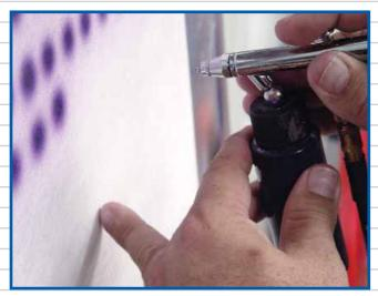
Fig 7: Use two hands for good control. I like to gently slide a free finger along the surface for consistency; it keeps me from getting too close. Just be careful of any wet paint!
